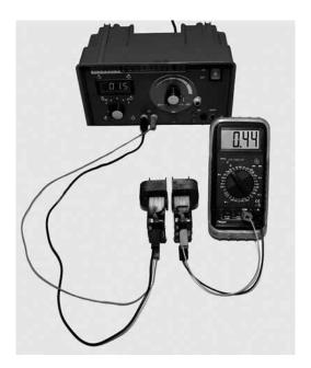
The student investigated the effect of inserting aluminium between the coils. The student inserted an aluminium plate in the gap between the coils and recorded the new reading V on the voltmeter. She repeated this for varying thicknesses t of aluminium.
